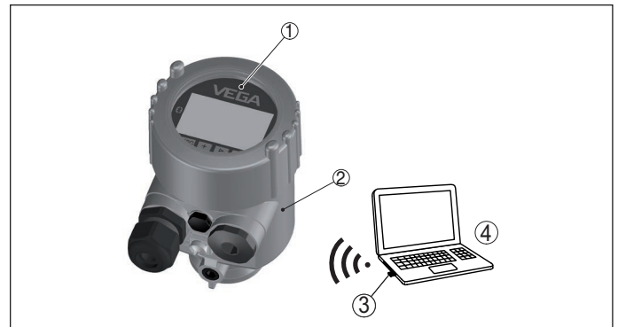
Fig. 29: Connection of the PC via Bluetooth adapter
