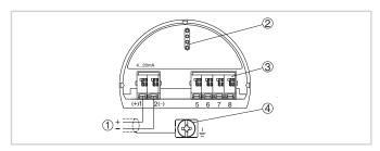
Electronics and terminal compartment, single chamber housing
