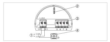
Electronics and terminal compartment, single chamber housing
