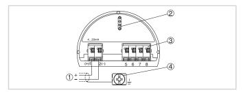
Electronics and terminal compartment, single chamber housing
