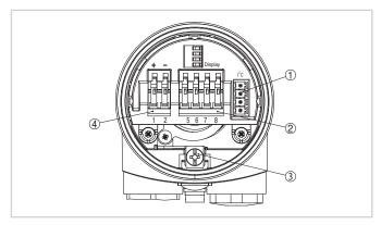
Electronics and terminal compartment, single chamber housing
